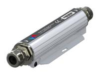
LZ PRO 01G-OT is a single-port surge protector designed for exterior applications with an IP 66 rated Aluminum alloy case. It supports 8 lines network signals and provides surge protection for wires. The maximum common mode surge voltage is 10KV(10/700us) and max differential mode surge voltage is 6KV(10/700us). It supports 10/100/1000Mbps of data rates. It well protects your device against surge damage.
